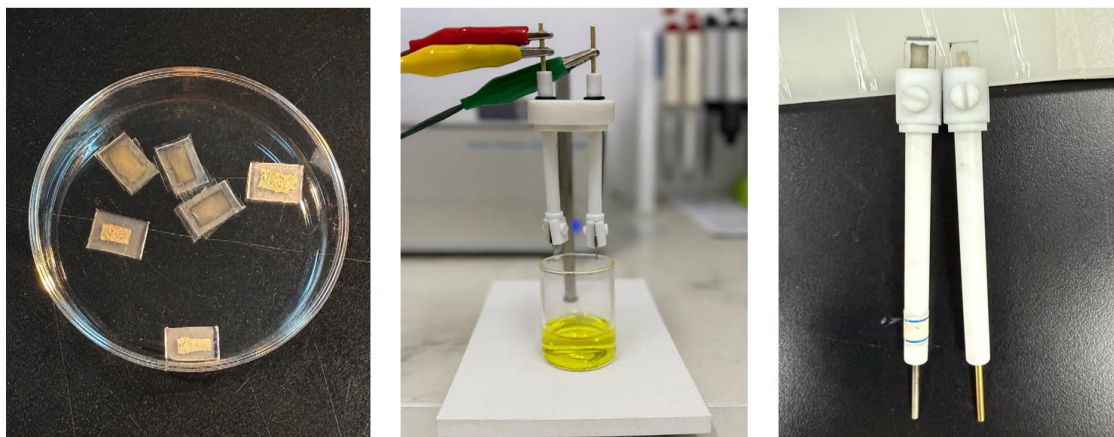
Figure 4 - Fabricated MXene/SiC-based conductive ink electrodes
