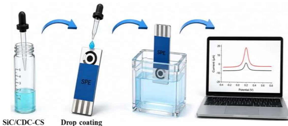
Figure 1 - Schematic illustration of the preparation of a SiC/CDC-CS/SPE and voltammetric detection of the analyte
