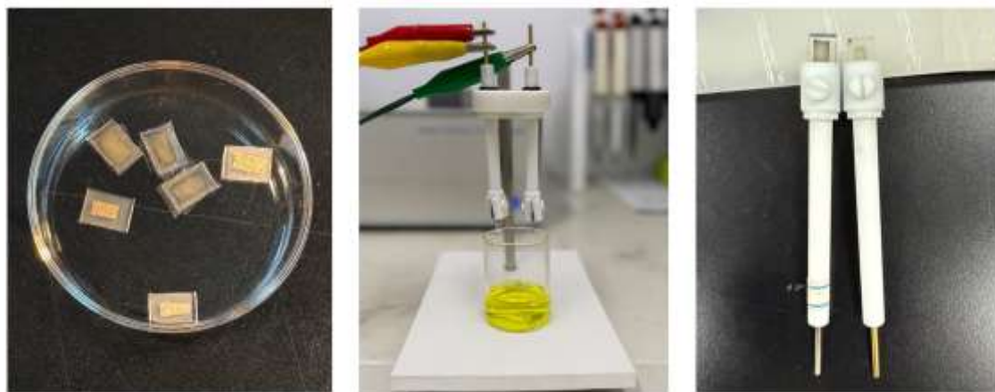
Figure 4 - Fabricated MXene/SiC-based conductive ink electrodes
