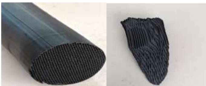
Figure 1 – Model filter made of carbon-silicon sorbent. a) Multichannel block end view b) Block in section
